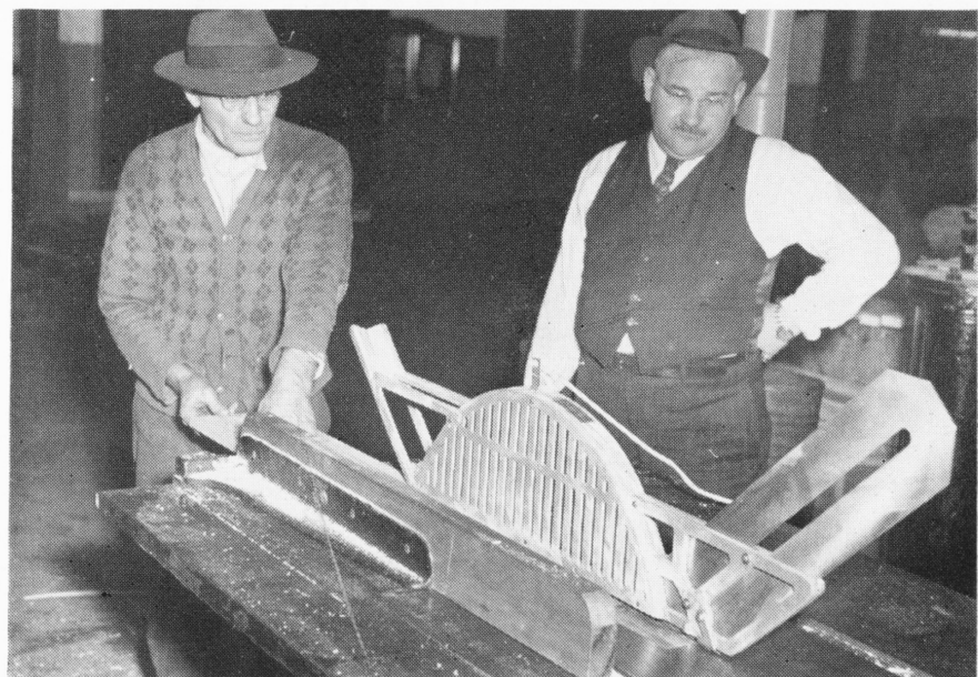
To Sam Boroch, right, and Phillip Schnell of the East Carpenter Shop, it's more than the latest type of saw guard they're looking over. As one of five new saw guards, it completes (yes, 100 per cent) the guarding of every piece of machinery in their department. Every possible effort is being made to guard employees from injury and if guard equipment is used properly, employees will rarely come within harm's reach.
